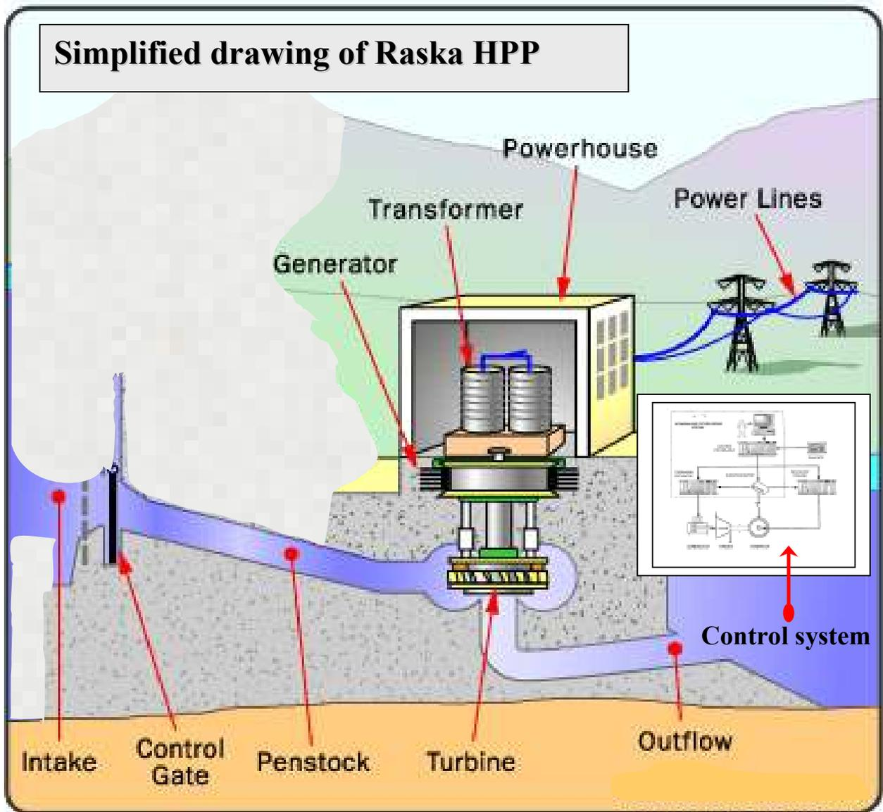
Figure 1. Simplified drawing of HPP “Raska”
