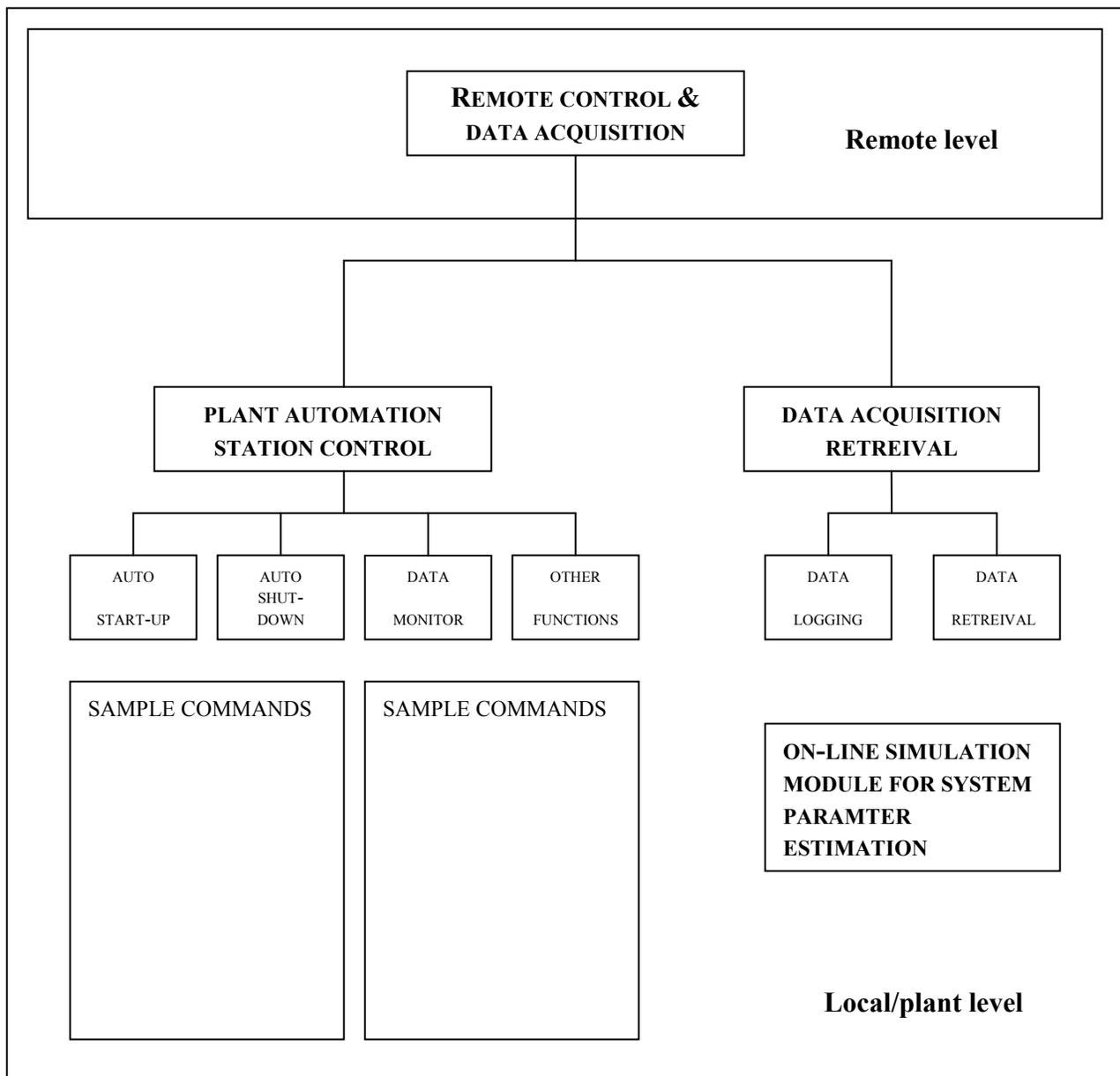
**Figure 3. Simplified overview of plant automatic control**
