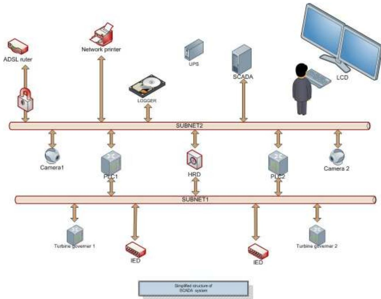
**Figure 2. Simplified structure of SCADA system**
