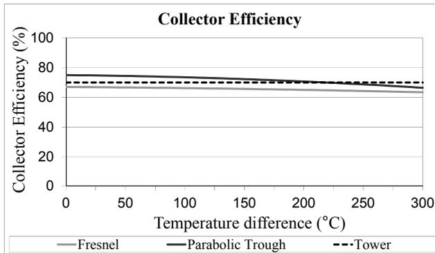
**Figure 10: Collector efficiency for different solar thermal technologies**
