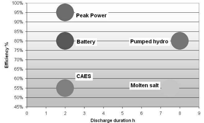
**Figure 5: discharge duration vs. efficiency of energy storage systems**
