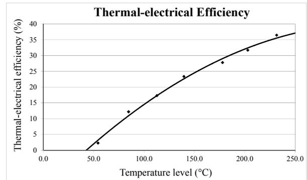
**Figure 11: Thermal-electrical efficiency evolution with the integration temperature**
