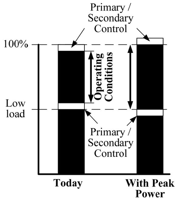
**Figure 6: Impact of Peak Power on the operating range of a Power Plant**
