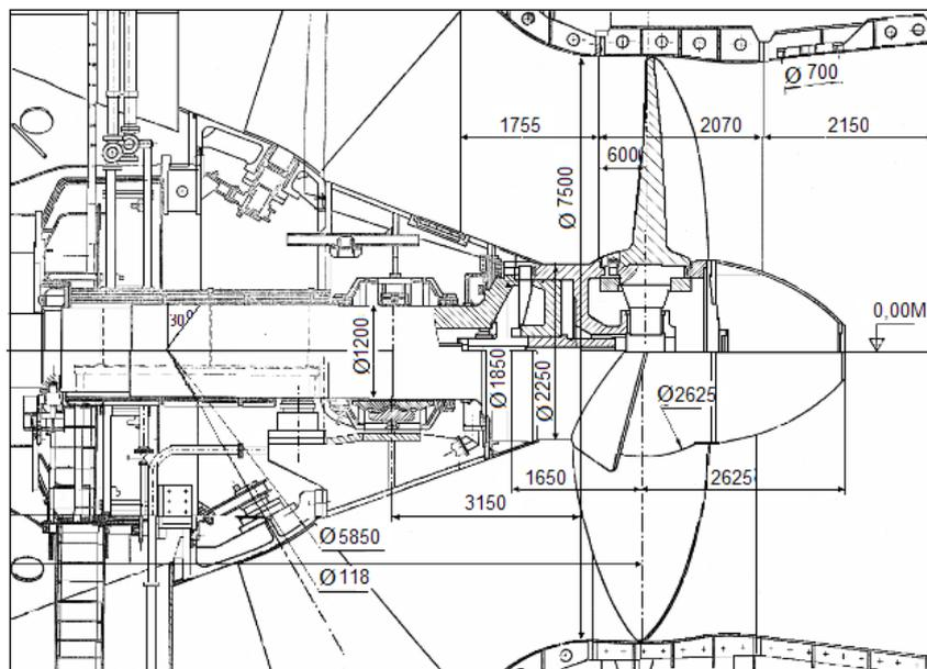
**Figure 1. Appearance of the Kaplan turbine, nominal power 28 MW**
