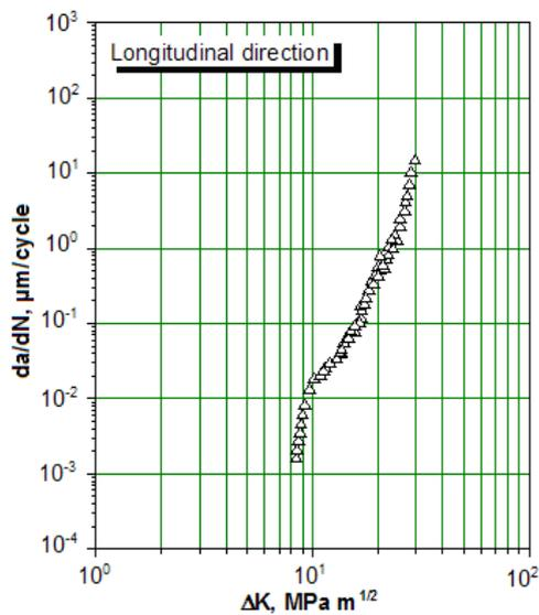
a) Longitudinal direction of the shaft flange casting
