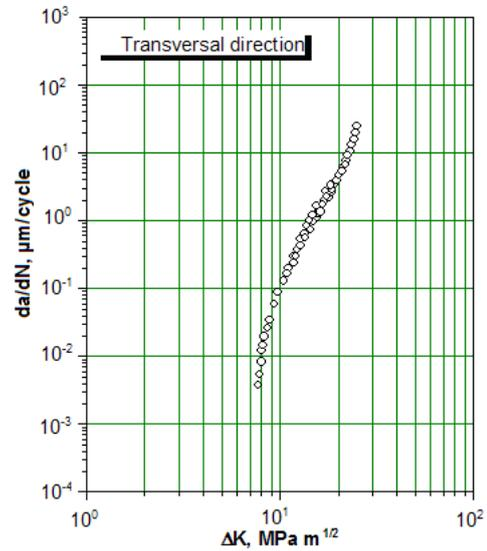
b) Transversal direction of the shaft flange casting
