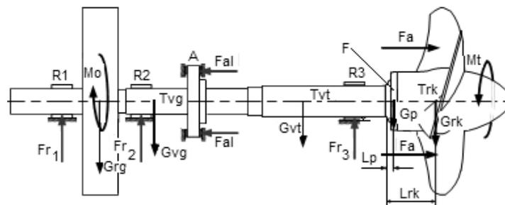
Figure 3. Turbine shaft with loads that occur on the hydro-electric generating set
