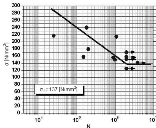
Figure 4. Dependency of fatigue strength  $\sigma$  on the number of cycles  $N$  (Wöhler's curve)
