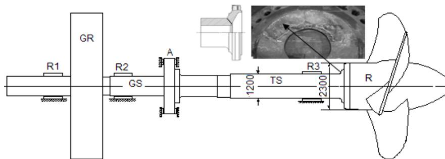
**Figure 2. Appearance of basic components of the generating, appearance of the fractured surface**
