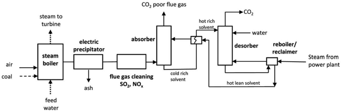
Scheme 6. Integrated system for post combustion CO<sub>2</sub> capture using amine washing
