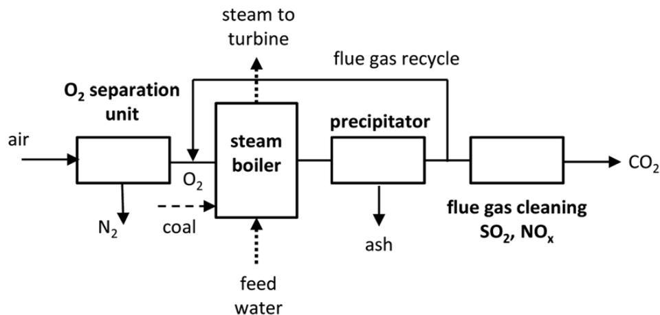
Scheme 4. Process scheme of CO<sub>2</sub> capture with oxyfuel combustion
